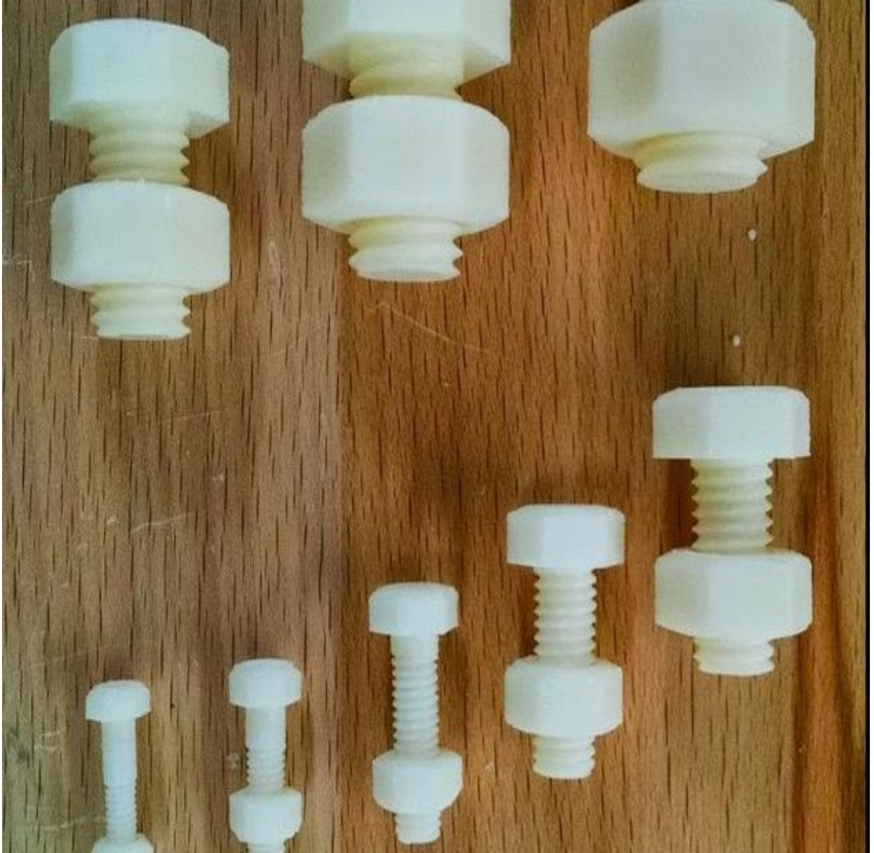
Figure 30 - 3D Printed Nuts and Bolts
